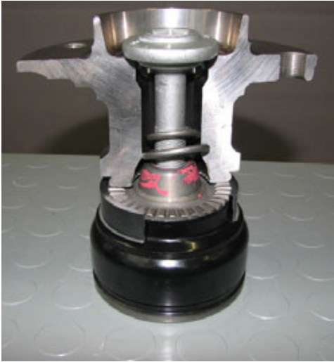
Cutaway view of the new front axle spur gear connection to the wheel hubs
